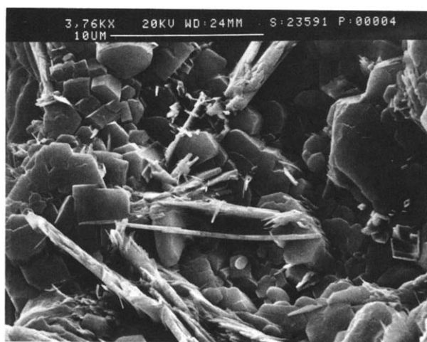
Fig. 7. SEM micrograph of the surface of V_2O_5 contaminated support treated for 3h at 1000 °C
